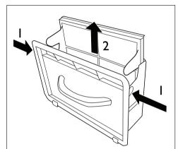
3. To clean the fluff filter: Remove filter from filter housing. To do this, press the pressure points on the sides and pull the filter frame up and out of the housing. Remove fluff from the fluff filter with a damp hand.
